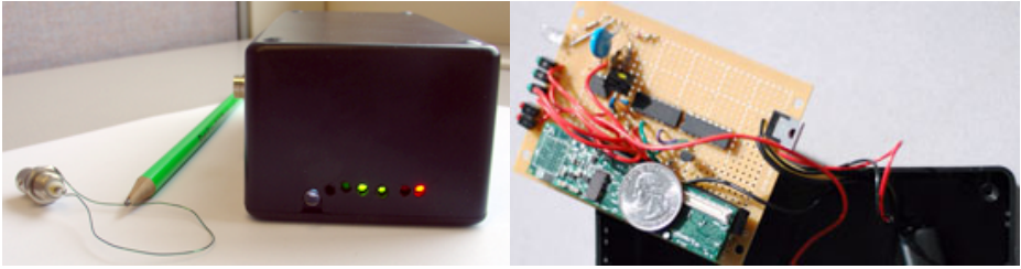
Fig. 1. Our assembled credit card emulator
